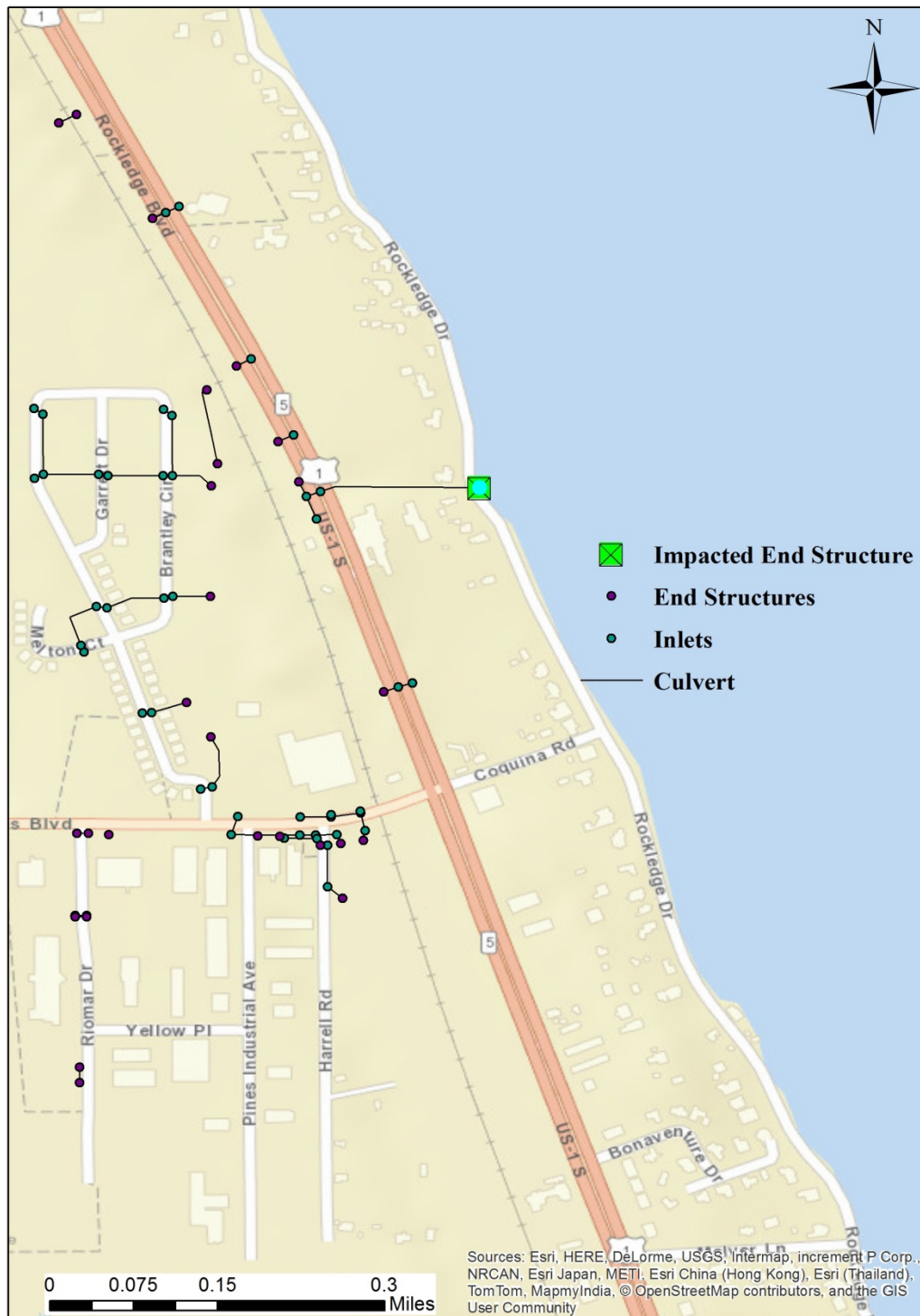
Figure 2b: Stormwater end structures showing potential top elevation inundation under 2020 annual high water (AHW) conditions, City of Rockledge (southern extent)
