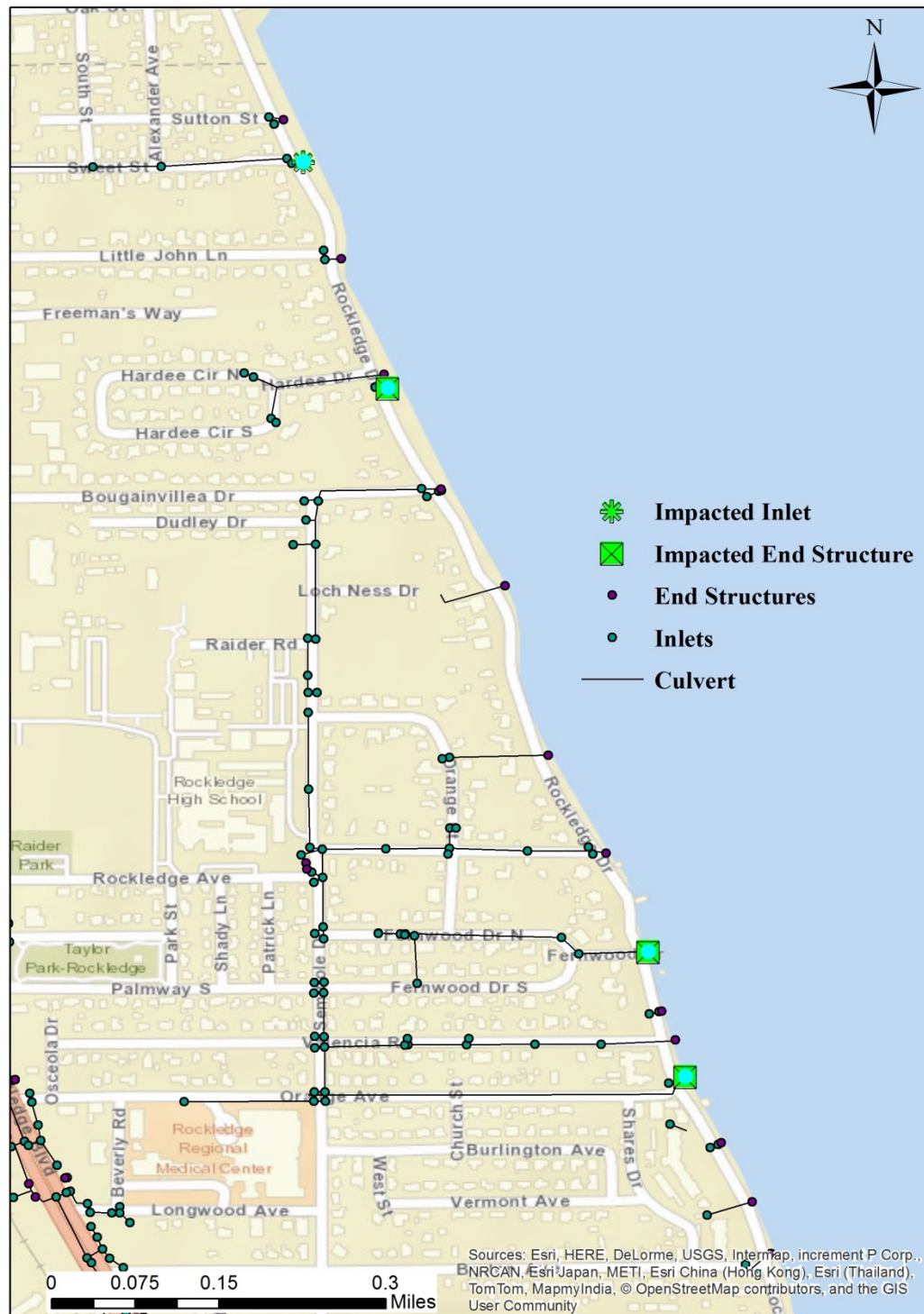
Figure 2a: Stormwater inlets and end structures showing potential top elevation inundation under 2020 annual high water (AHW) conditions, City of Rockledge (northern extent)
