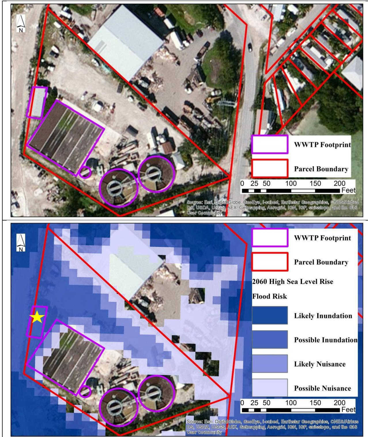
**Figure 8: Key Haven Wastewater Treatment Plant.** Aerial photograph (top) and 2060 high sea level rise assessment (bottom). Yellow star indicates structure with flood risk.
