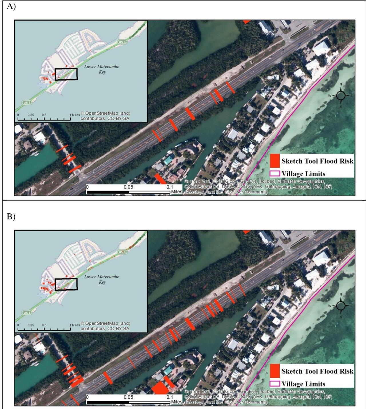
**Figure 16b: FDOT Sea Level Rise Sketch Planning Tool Close-Up for US1, Lower Matecumbe Key, 2060 Sea Level Rise Scenarios.** Picture A) shows road segments predicted as vulnerable to nuisance flooding with 9 inches of sea level rise (2060, Low Scenario). Picture B) shows road segments predicted as vulnerable to nuisance flooding with 24 inches of sea level rise (2060, High Scenario).
