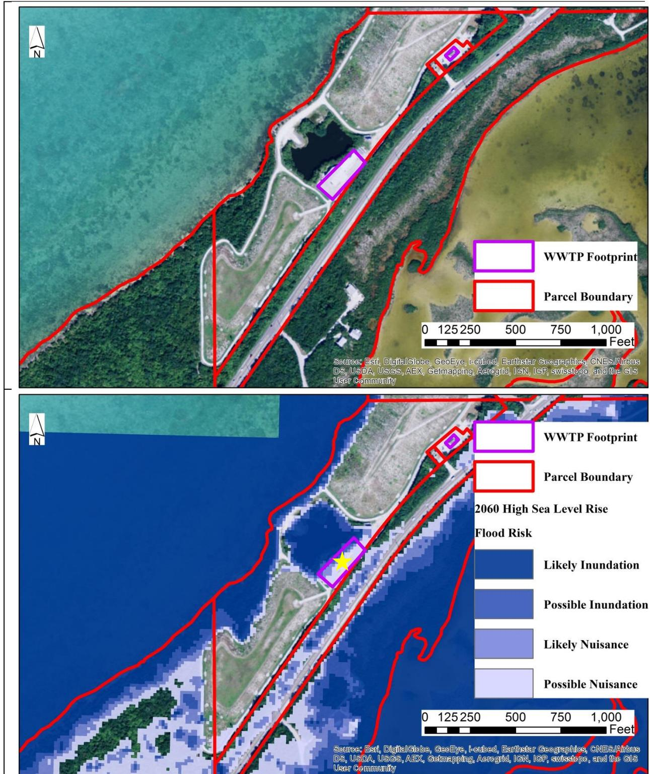
**Figure 13: North Key Largo Wastewater Treatment Plant.** Aerial photograph (top) and 2060 high sea level rise assessment (bottom). Yellow star indicates structure with flood risk.
