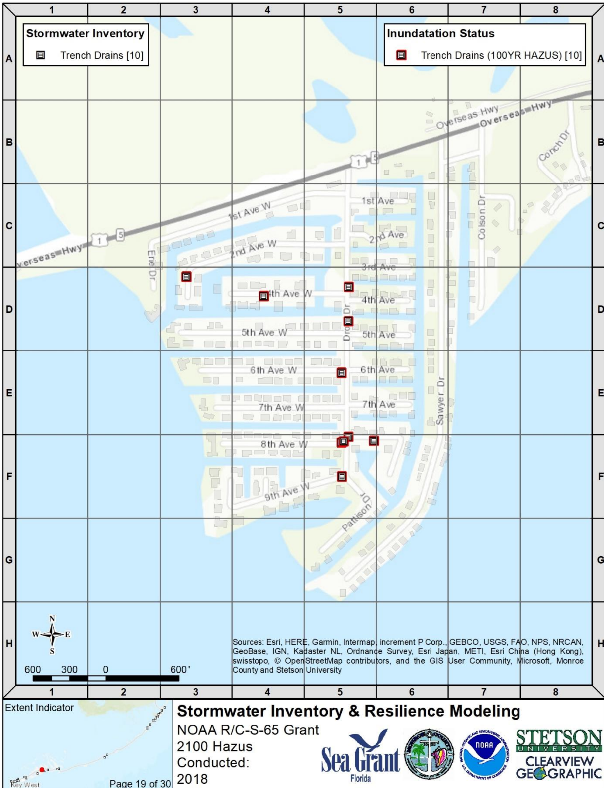
Map Series 6: Monroe County Stormwater Infrastructure Inventory with Potential Future Vulnerability to Hazus-MH 100-Year Coastal Flood, 2100 Intermediate-High (4.13') Sea-Level Rise
