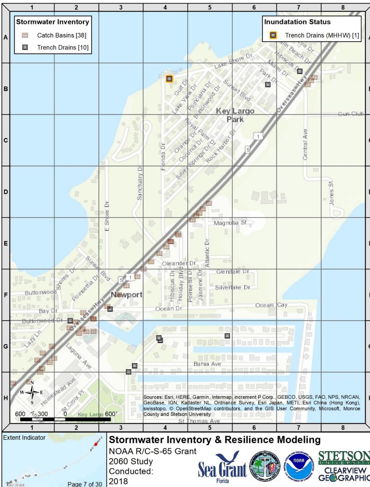
Map Series 3: Monroe County Stormwater Infrastructure Inventory with Potential Future Vulnerability to Tidal Flooding, 2060 Low (14") and 2060 High (26") Sea-Level Rise
