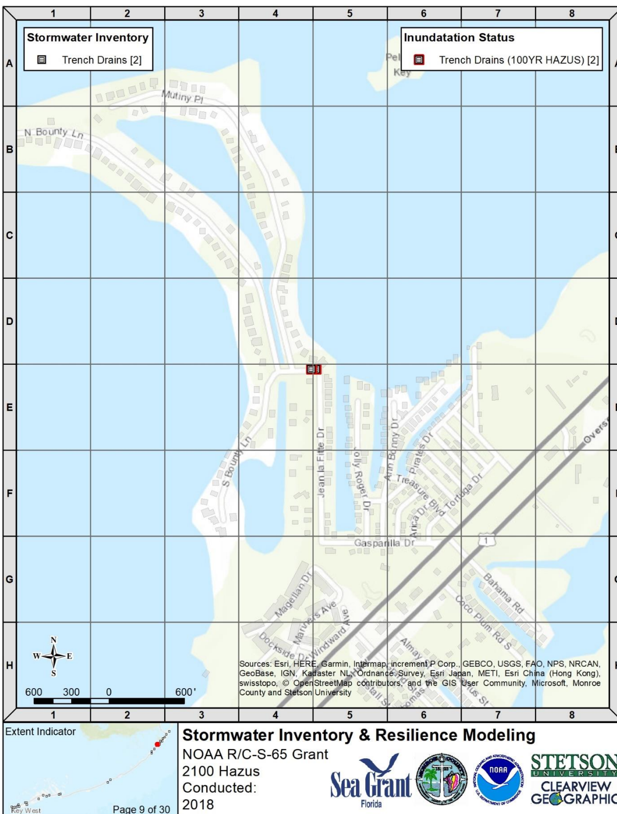
Map Series 6: Monroe County Stormwater Infrastructure Inventory with Potential Future Vulnerability to Hazus-MH 100-Year Coastal Flood, 2100 Intermediate-High (4.13') Sea-Level Rise
