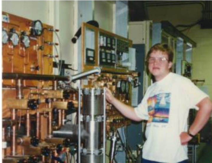
Figure 3 Garrett checking the controls of the Cryo-2 microKelvin cryostat during a Liquid He transfer. University of Florida MicroKelvin Facility, 1996.
